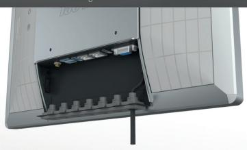
An important novelty is also innovative cable management, so that the user can easily and at any time reach the connectors, connect only the cable that he really needs and that the cable connection has IP protection.
