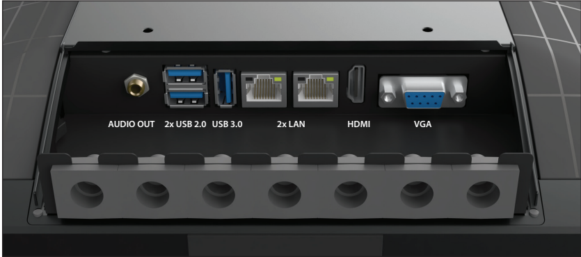
Figure 7.2 Connectors of Uniq PC II Celeron J1900
