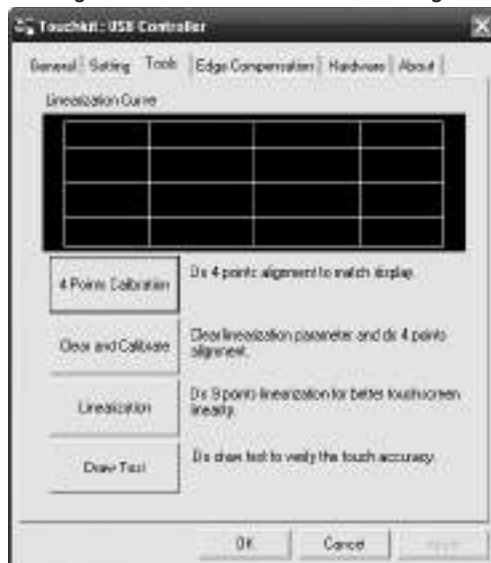
Figure 2.3. Tab for the calibration settings
