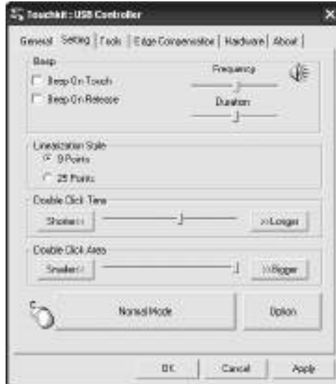
Figure 2.6. Tab for other settings of the touch screen display
