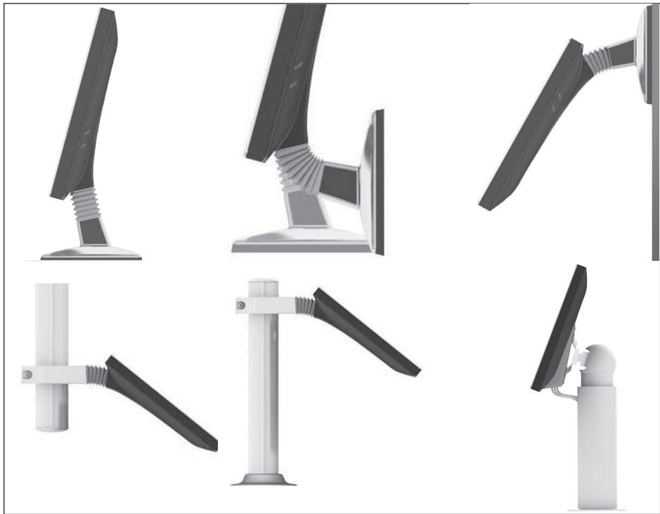
*Note: For placing a Uniq Display on a wall it is possible to achieve a larger angle of the display tilt by rotating its leg by 180°. Only an ELCOM service center is authorized to perform this operation.*
