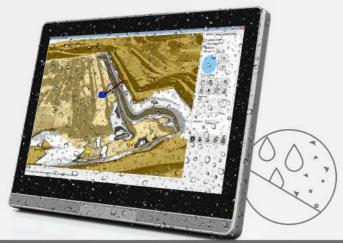
Robust and waterproof construction with protection class IP65 safely resists dust, shocks and immersion in water
