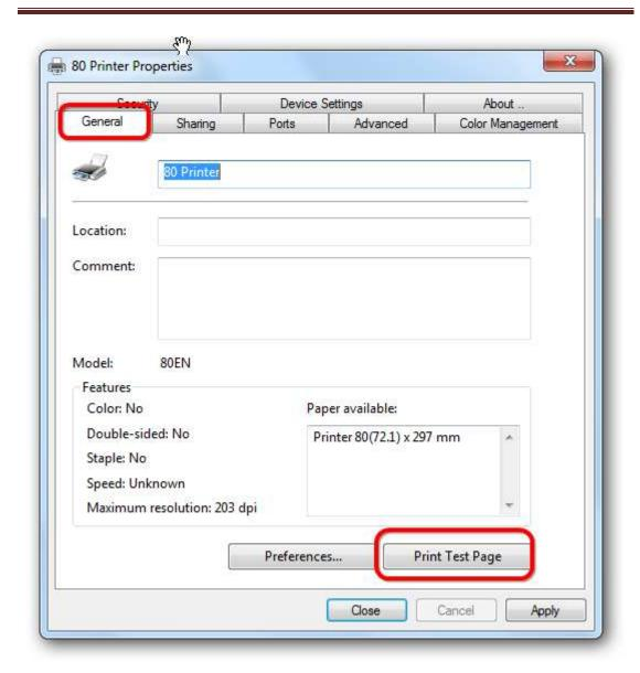
Click "Print Test Page", the printer will print test page, which means the printer has been connected with computer successfully and the port configuration is correct.
