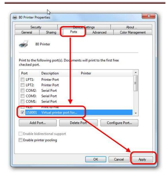
Select available computer USB communication port, such as the above picture shows "USB001", and then click "Apply" to finish the configuration.
