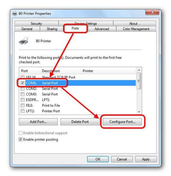
Select available computer COM port, such as "COM1" as the above picture, and then click "Configure Port" to set the detailed parameter.
